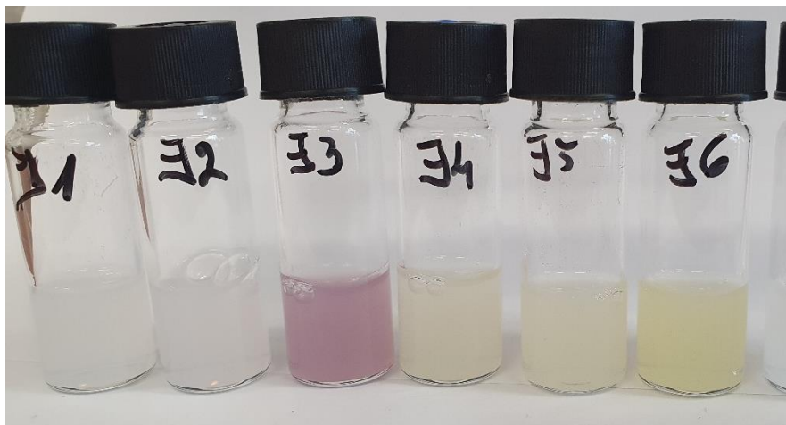
Figure 3.12 shows the BSA/Au bioconjugate /PNIPAAm-co-Ala samples in water after one days from preparation
